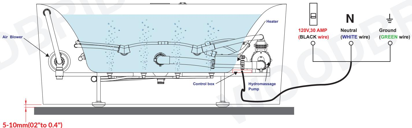
1. **IMPORTANT!!** Every electronic device has induced current, and it is a MUST to add a ground wire connection.
