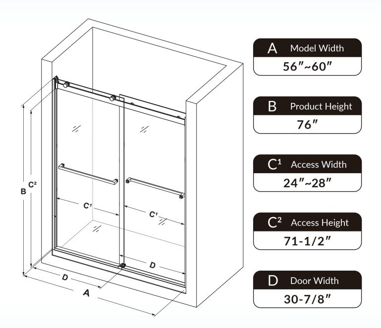
Glass Thickness: **5/16"(8mm)** Minimum Threshold Required: **3"**
