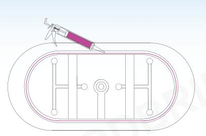
6. Apply a generous bead of adhesive or waterproof silicone to the bottom of the tub and a bead of tub and tile caulk around the edge of the tub
