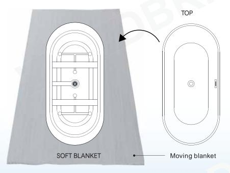
2. Turn bathtub upside down and set it on a non-abrasive mat, blanket, or cardboard to prevent any scratches on tub rim.
