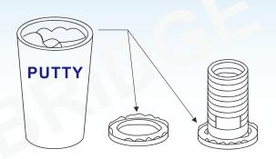
6. Install 1 <sup>1</sup>/<sub>2</sub>" rubber slip gasket over the drain waste vent.
