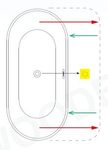
1. Clean, level and prepare the floor for installation, Place the tub in the exact installed location on the floor and trace the outline of the bathtub with pencil and mark the drain hole location on the floor. Move the tub away so that the plumbing can be installed.
