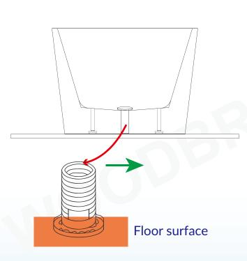
5. Clean the surrounding of the drain pipe with cloth in preparation of setting the drain, the area should be dry and free of any debris. Apply a bead of clear silicon or plumber putty around the drain body and pass it through the drain hole, also apply plumber putty to the washer and slide it over the bottom of the drain body.
