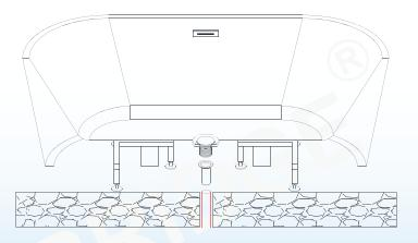
8. Flip the tub over and carefully set the tub into position with tail piece assembly to waste vent and connect to the drain.
