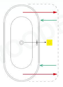
1. Clean, level and prepare the floor for installation, Place the tub in the exact installed location on the floor and trace the outline of the bathtub with pencil and mark the drain hole location on the floor. Move the tub away so that the plumbing can be installed.
