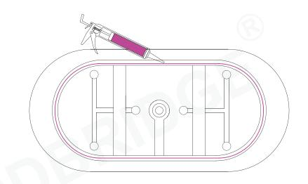
7. Apply a generous bead of adhesive or waterproof silicone to the bottom of the tub and caulk around the edge of the tub.
