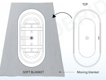
2. Turn bathtub upside down and set it on a non-abrasive mat, blanket, or cardboard to prevent any scratches on tub rim.
