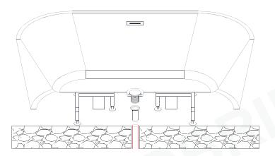
7. Flip the tub over and carefully set the tub into position with tail piece assembly to P-trap and connect to the drain.
